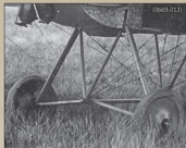
Undercarriage detail from early production Fokker E.1 13/15 D showing strut fairings and rigging.
