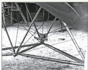
Undercarriage detail and wing warping cable rigging detail from a Fokker E.IV thought to be 638/15. Although this is a Fokker E.IV the details shown here are pertinent for the Fokker E.1.
