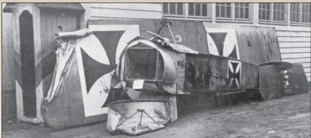
Another unidentified early production Fokker E.1 awaits repair. Although the shortened aluminium side panel confirms this is an early production aircraft the wings appear to be the longer 13 rib 10.05m wingspan types usually associated with later production Fokker E.1 (and E.II, E.III & E.IV).
